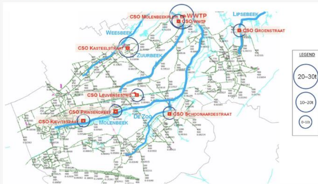
Figure 10. Example of GIS-based reporting: map of Kortenberg catchment including sewer system (green), receiving watercourses (blue), and locations of major emission points from urban wastewater system (red: WWTP and main CSOs). Circles indicate the magnitude of emitted annual loads (in tons).
